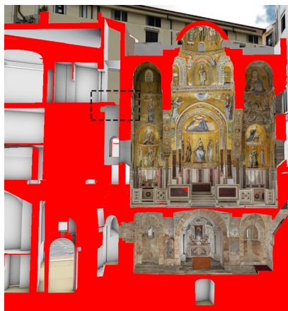
Figure 10 Cross-sections of the Royal Palace and the Cappella Palatina in Palermo; left: three-dimensional model; right: AutoCAD output. The black dashed boxes indicate the 1585 slabs of the modern courtyard (Cortile della Fontana), formerly supported by vaults, which obliterated the original openings on the North side of the Cappella Palatina sanctuary. Graphic: TecnoArt; © A.R.S. 2015.
